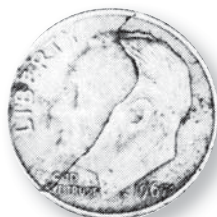
Lamination crack III-D-1
