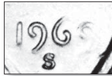
Struck through a filled die III-K-4
