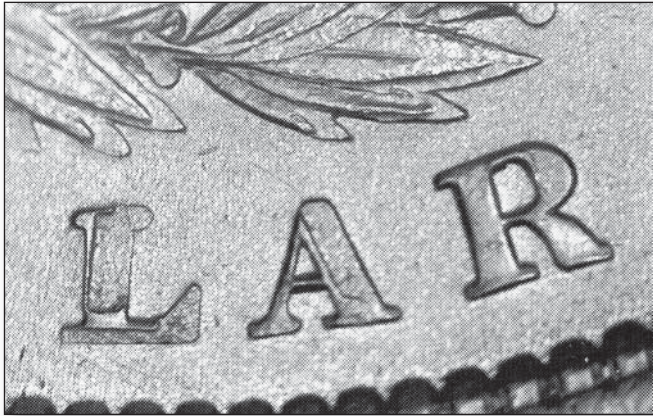
Machine doubling damage V-B-1
