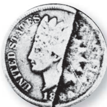
Layer peeled off III-D-2
