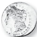
Struck off center 10 to 30 percent III-M-7
